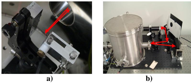
**Figure 2.** Membrane clamped in the vice inside the inner experimental chamber (a). Detection of the reflected beam (b)
