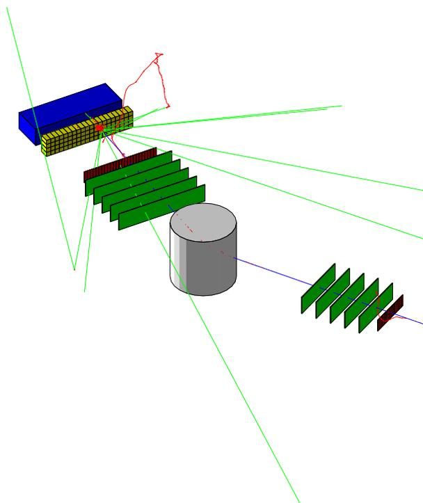
Fig. 5. DAWN view of demonstration detector with trajectories.
