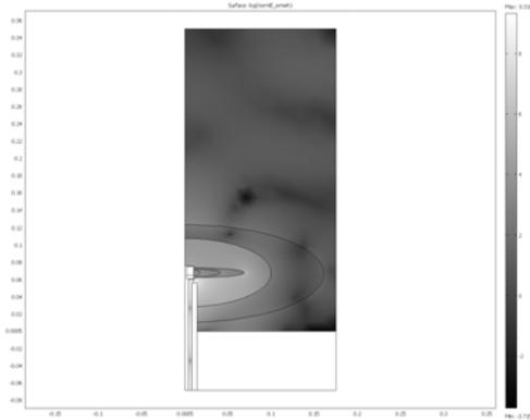
**Figure 8.** Variations of  $\log(\text{norm}(E))$  inside the plasma chamber, in vacuum (2.45 GHz). Dipolar source is located at the bottom and the symmetry axis is on the left. Five elliptical shape areas are arbitrary defined around the dipolar source.
