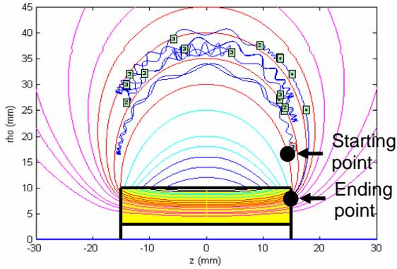
**Figure 10.** Electron trajectories around a cylindrical magnet of 30 mm in length and 20 mm in diameter. Electron energy is 20 eV distributed randomly over the three components ( $v_x$ ,  $v_y$  and  $v_z$ ).
