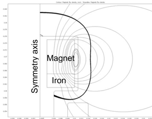
**Figure 4.** Magnetic field lines, thin lines and line of constant intensity (875 G) in bold line for a magnet of 10 mm height and 20 mm in diameter. An additional part, 4 mm thick of ARMCO iron, is placed at the magnet bottom.
