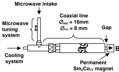
**Figure 1.** Sketch of the dipolar microwave (2.45 GHz) plasma source. A source consists of a tuning system, a coaxial line (partially under vacuum) and a cooled permanent magnet with an axial  $\mathbf{B}$  field.
