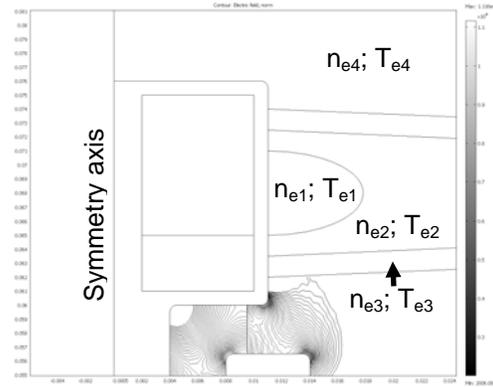
**Figure 9.** Close view of  $\text{norm}(E)$  (iso-values) around the dipolar source with plasmas zones. Plasma parameters density and temperature (respectively  $n_e$  and  $T_e$ ) are constant in each zone.
