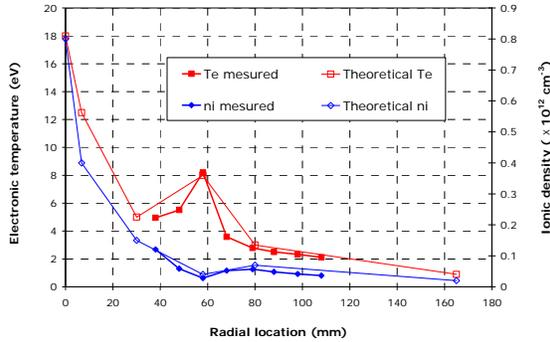
**Figure 7.** Radial variations (from the magnet's surface) of plasma density ( $n_i$ ) and electron temperature ( $T_e$ ) in the mid-plan of the magnet. Experimental data are in filled spots and data used in the model are represented in unfilled spots.
