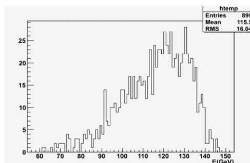
Figure 1: Energy distribution of disrupted beam particles lost at the first collimator QEX1COLL, located at 45 m from the IP.
