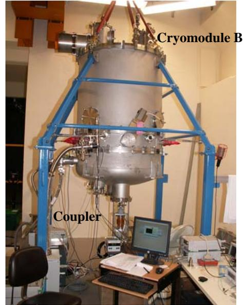
Figure 11: Coupler mounted on the cryomodule B.
