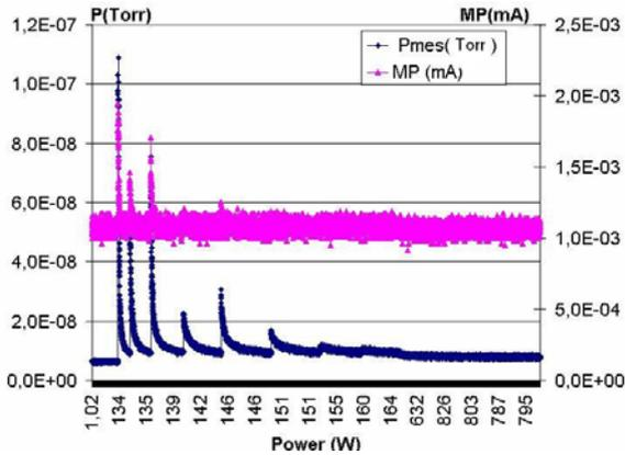
Figure 9: Multipacting and vacuum measurement versus RF power
