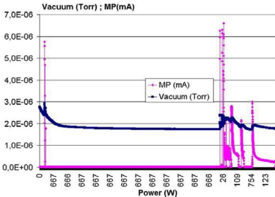
Figure 10: Multipacting and vacuum measurements versus the RF power.
