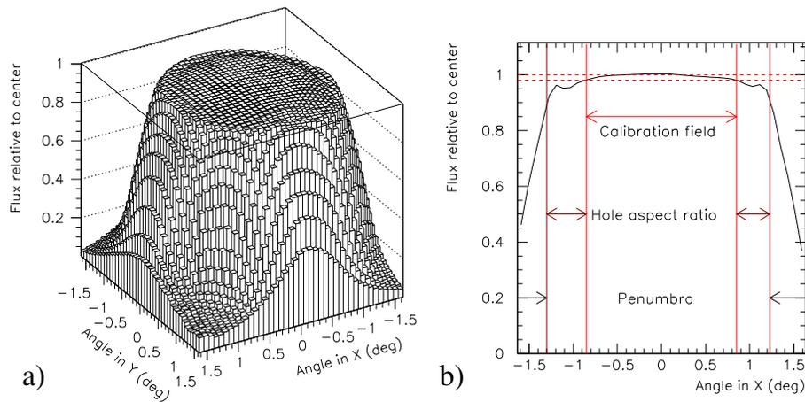
Figure 5: a.)XY scan of the illumination field of the LED light source in Figure 4. The photocurrent measured in the central flat field, generated by a  $5.8 \text{ mm}^2$  photodiode at 0.9 m, is about 12 pA. b.) A cut of this field along a symmetry axis shows a  $\pm 0.8^\circ$  calibration field with a  $\pm 1\%$  uniformity, surrounded by a rougher region of  $0.4^\circ$  due to a bad aspect of the angular diaphragm and a penumbra zone.
