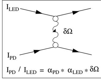
Figure 7: LED and photodiode quantum efficiencies.
