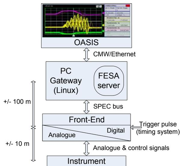
Figure 1 System architecture
