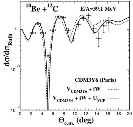
Fig. 3. Cross sections for the  $^{10}\text{Be} + ^{12}\text{C}$  elastic scattering at 39.1A MeV are compared with calculations using the CDM3Y6 folding potential and the imaginary potential  $W$  (dashed line). Data are better reproduced taking into account a complex VCP  $U_{VCP}$  (solid line), given in the text.
