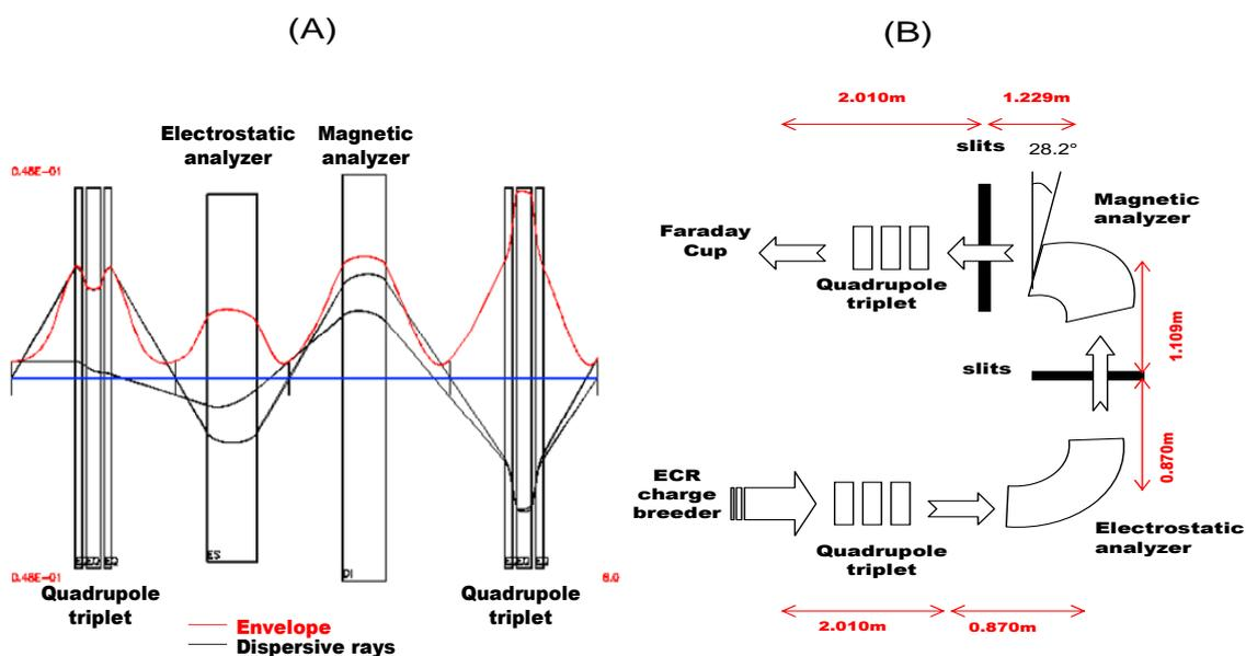
**Figure 4:** (A) Simulations of the beam envelope through the isotopic separator in the dispersive plane with COSY INFINITY. (B) Preliminary sketch of the separator setup with the calculated relative distances.
