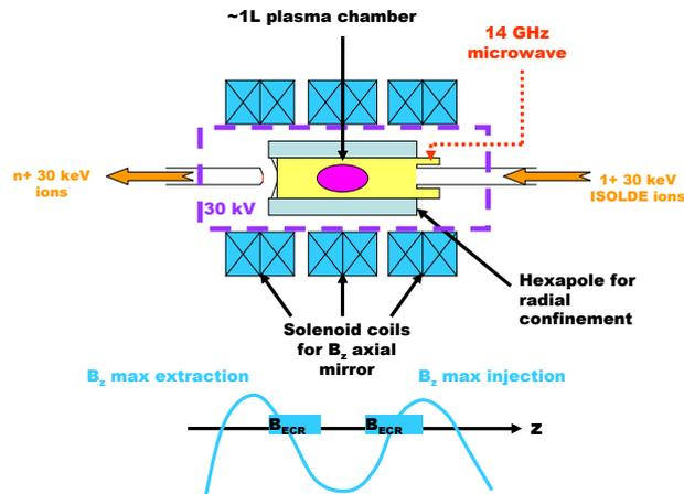
**Figure 1:** Ion motion inside the ECR charge breeder: the  $1+$  ions are stopped and then ionized in the plasma. The plasma is trapped in a configuration where the axial magnetic field  $B$  shows a minimum.
