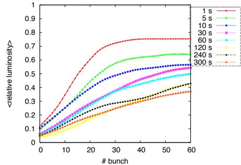
Figure 3: Beam-based IP position feedback simulation for the  $e^+e^-$  collision with ground motion model B applied for successive time intervals along the BDS. The average relative luminosity is calculated over 50 seeds.
