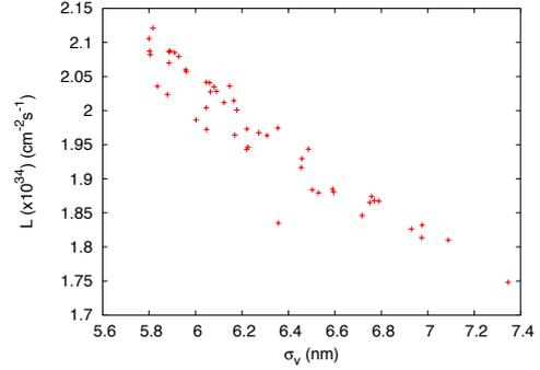
Figure 6: Luminosity versus the combined vertical beam size of both  $e^-$  and  $e^+$  beams at the IP. Feedback simulation carried out for  $e^+e^-$  collisions under the effect of the missalignments produced by the ground motion after 1 s.
