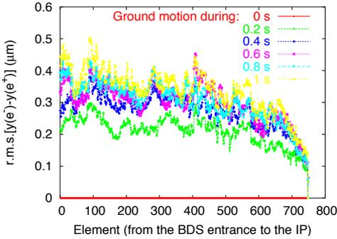
Figure 2: Difference in misalignment of each BDS element in the  $e^-$  line with respect to the same element in the  $e^+$  one. Ground motion model B was applied at successive time intervals. The results are the *r.m.s.* of 50 seeds.
