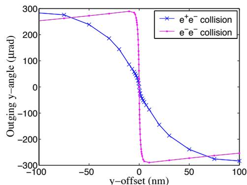
Figure 1: Vertical deflection angle versus vertical half beam-beam offset, for  $e^+e^-$  and  $e^-e^-$  collisions simulated with GUINEA-PIG [3], using ideal Gaussian beam distributions with ILC nominal parameters at 500 GeV in the center-of-mass [4].
