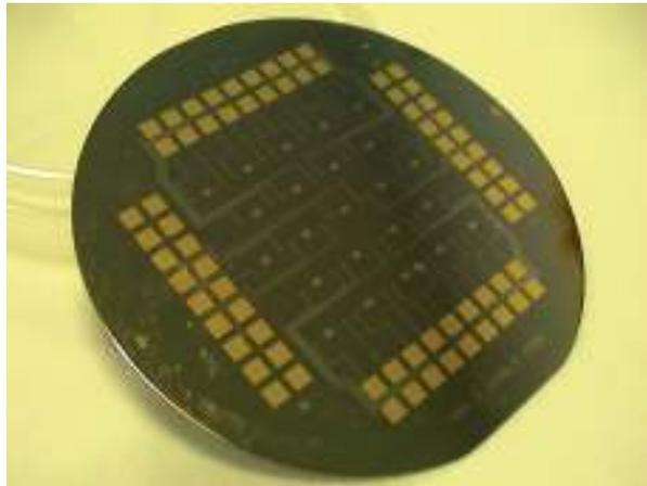
Fig. 3: (color online) 23 pixels thermometers only array
