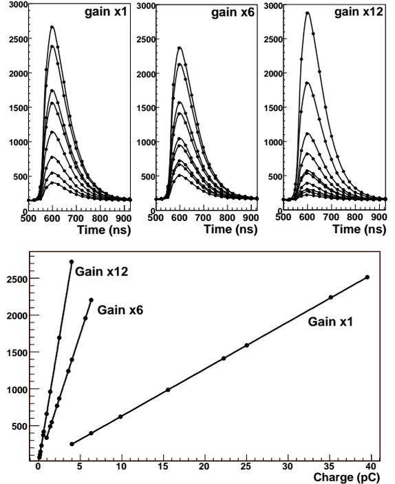
Figure 1. Top: Pulse shapes of VFE output Lines are to guide the eyes. Bottom: VFE output in ADC counts versus injected charge
