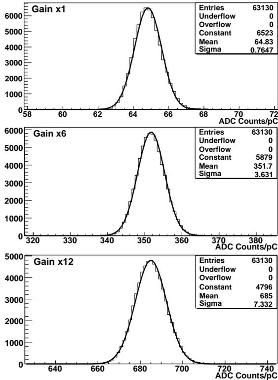
Figure 2. Slope distributions of the injected charges versus pulse height in ADC counts/pC.
