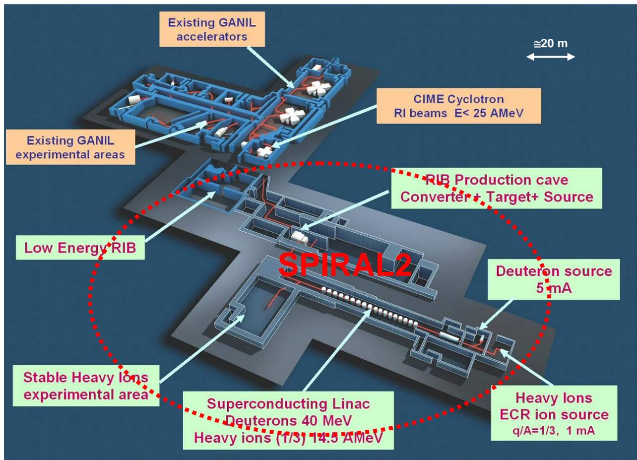
Figure 1 : Layout of the SPIRAL2 accelerator complex
