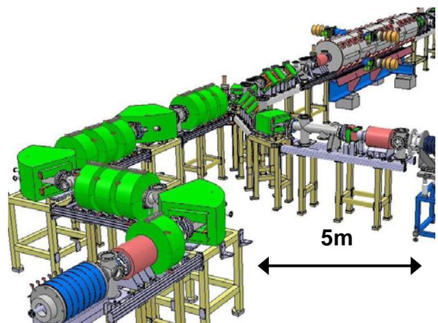
Figure 2: Layout of the injector beam lines
