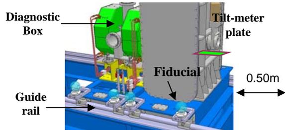
Figure 10: Cryomodule A and quadrupoles fiducialization
