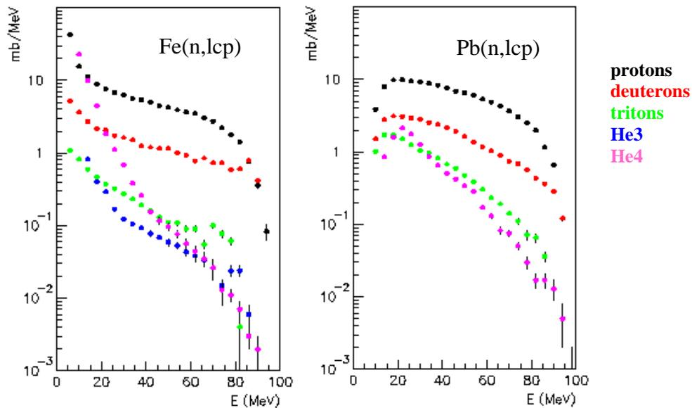
Figure 2: Energy-differential cross sections for the emission of light-ions induced by 96 MeV neutrons on  $^{\text{nat}}\text{Fe}$ ,  $^{\text{nat}}\text{Pb}$ .
