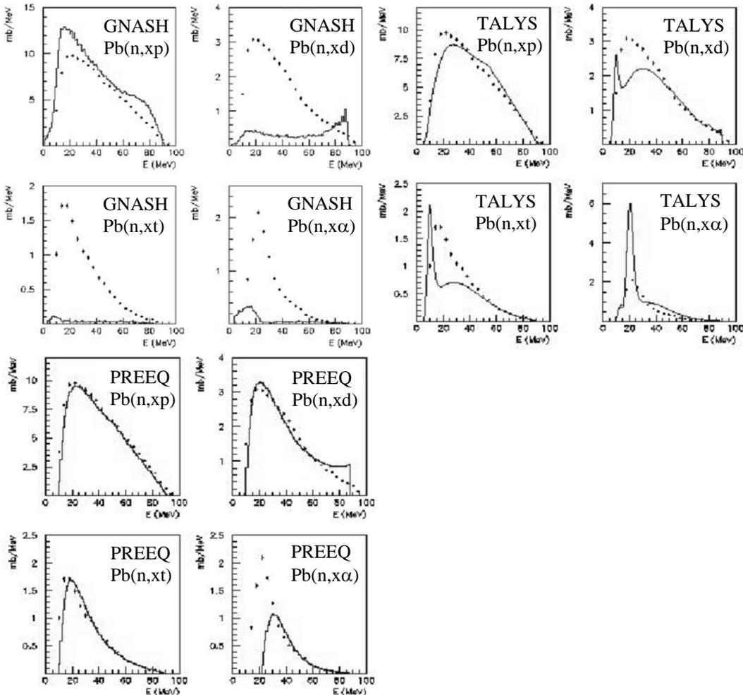
**Figure 3:** Energy-differential cross sections calculated using the GNASH, TALYS and PREEQ codes. The calculations have been done for 96 MeV neutrons on Pb and are shown as histograms. The experimentally obtained data are shown as points.
