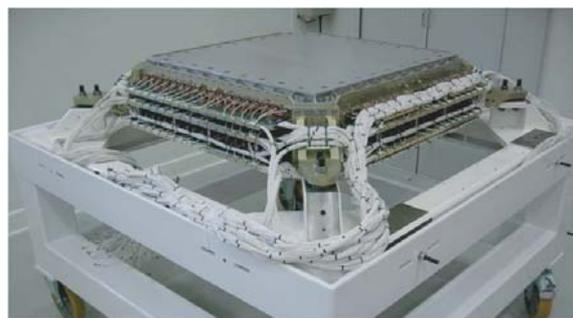
**Figure 3.** The calorimeter fully equipped with front-end electronics.
