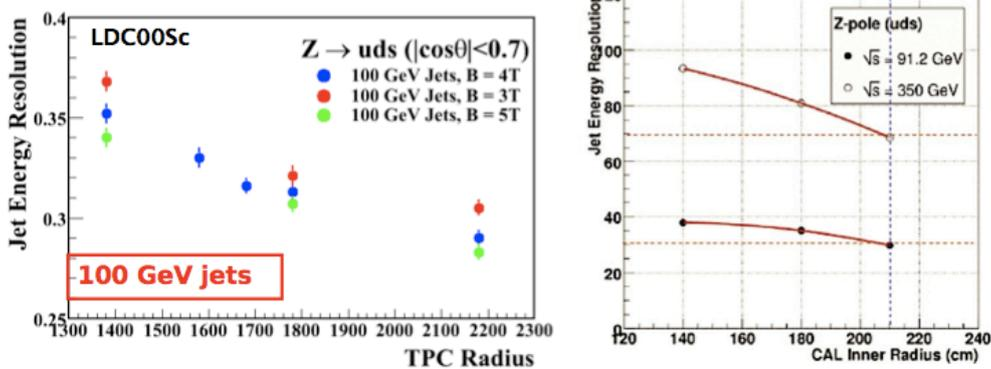
Figure 3: Examples of results of detector optimization studies within the MARLIN (left) and URANUS framework (right).
