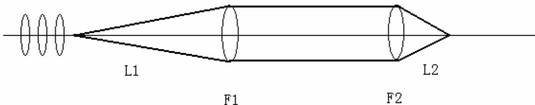
Figure: 1 A one-dimensional telescopic system.
