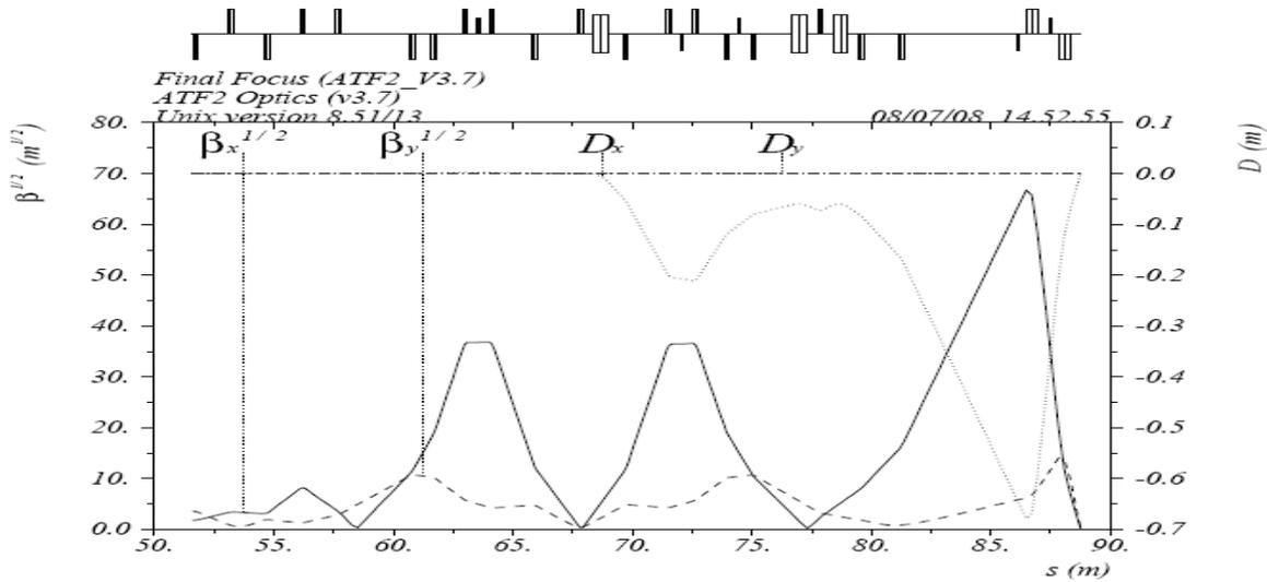
Figure 6:  $\beta$  functions with nominal  $\beta_x$  and twenty times  $\beta_{y,nominal}$  at the waist at -54cm.
