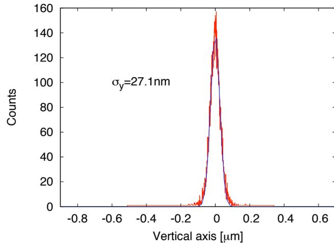
Figure 2: Vertical beam distribution at the IP for a preliminary optics with a factor 4 reduction in  $\beta_y$ . Aberrations and/or optics still need optimization for this pushed option since the ideal beam size would be  $\sigma_y = 17\text{nm}$ .
