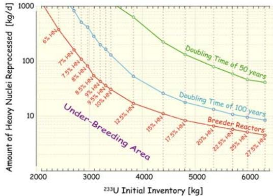
Fig. 4. Amount of heavy nuclei reprocessed per day versus initial fissile ( $^{233}\text{U}$ ) inventory, for different heavy nuclei proportions in the fuel
