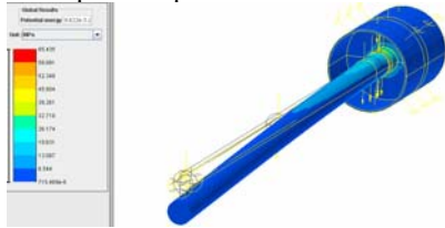
Figure 10: Stress of the coupler in the transports at 10g
