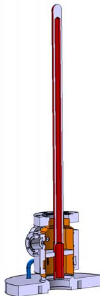
Figure 7: Updated design of the RF coupler.
