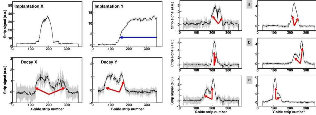
Fig. 4. Left: the upper part shows the energy signal for  $X$  and  $Y$  strips for a  $^{45}\text{Fe}$  implantation event; the lower part shows the energy signals for the subsequent 2-proton decay: the arrows represent the particles movement in  $X$  and  $Y$  directions, and the protons are emitted from the place where the ion was stopped. Right: other examples of energy signals for 2-proton decay events after  $^{45}\text{Fe}$  implantations (not shown here).
