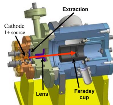
Figure 8: Setup for calibrating the alkali ion gun
