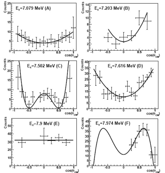
FIG. 2: Center-of-mass angular distributions measured for each excited state in  $^{19}\text{Ne}^*$ . Lines correspond to the best fits obtained in the present analysis. Part of the angular distribution of levels E and F was beyond the angular coverage of the detectors.
