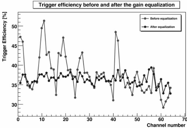
Fig. 9. Trigger efficiency as a function of channel number before and after gain equalization.
