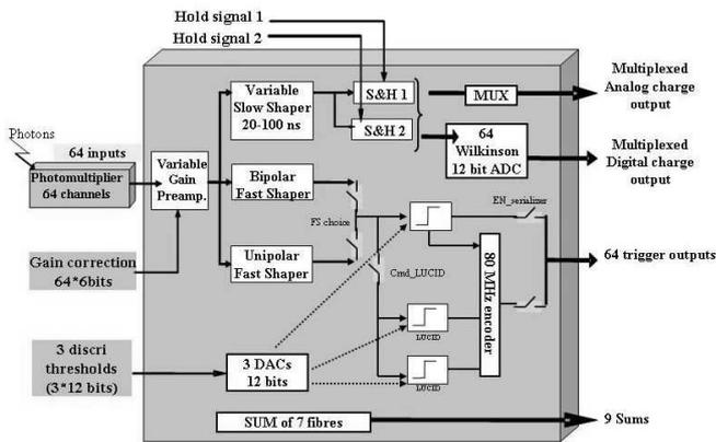
Fig. 6. Block diagram of MAROC second version.
