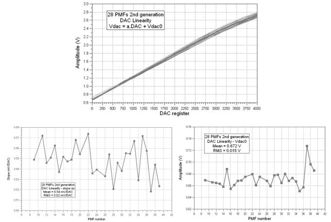
Fig. 11. Top: DAC linearity for the 28 active boards. Bottom left: slope of the DAC linearity fit as a function of PMF number. Bottom right: intercept ( $V_{dac}$  at  $DAC=0$ ) of the DAC linearity fit as a function of PMF number.
