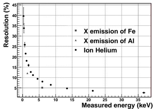
**Fig. 1.** Energy resolution ( $\sigma/E$ ) of our TPC for a  $^4\text{He}$  recoil in an 95%  $^4\text{He}$  + 5% Isobutan mixture at 700 mbar. X emission from  $^{55}\text{Fe}$  and  $^{27}\text{Al}$  are also shown.
