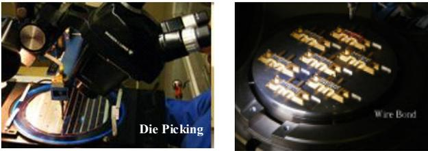
Figure 3 : manufacturing phases
