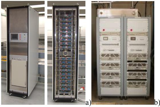
Figure 19 : a) Eurisol 10 kW (352 MHz) and b) Spiral2 20 kW (88 MHz), CW, power amplifiers.
