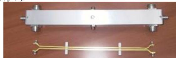
Figure 13 : coupled line combiner (© DB Elettronica)
