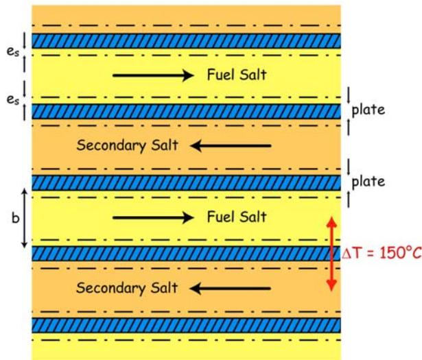
**Fig. 3** Partial schematic vertical section of the plate heat exchangers, the blue striped areas representing the plates. The temperature differential of 150°C between the primary and the secondary coolants is indicated.
