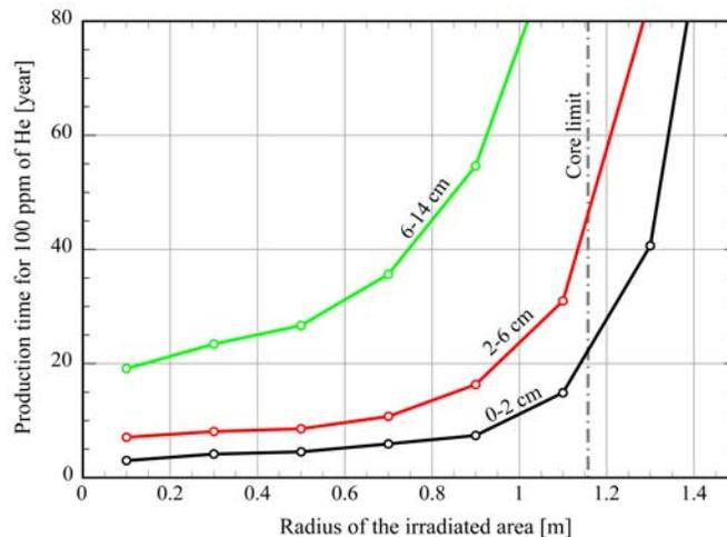
**Fig. 7** Operation time necessary to produce 100 ppm of He in different depths of the axial reflector, as a function of the irradiated area considered (zero corresponding to the centre of the core), with a fuel salt volume of  $18 \text{ m}^3$
