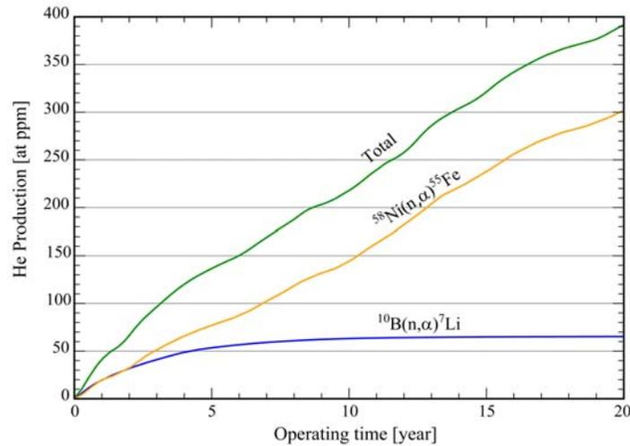
**Fig. 6** Contributions of the different nuclear reactions involved in Helium production in the most irradiated part of the axial reflector (radius 20 cm and thickness 2 cm), as a function of the reactor operating time, for a fuel salt volume of  $18 \text{ m}^3$
