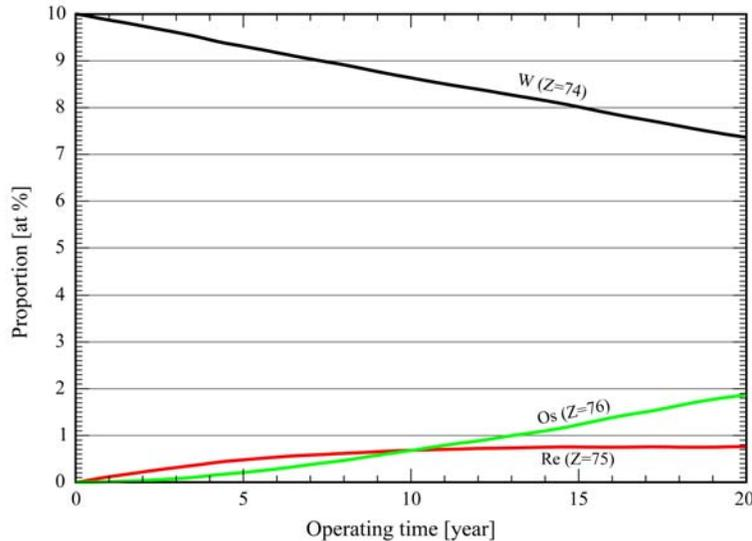
**Fig. 9** Contents in Tungsten (W), Rhenium (Re) and Osmium (Os) of the most irradiated part of the axial upper reflector (central area of radius 20 cm and thickness 2 cm), with a fuel salt volume of 18 m<sup>3</sup>
