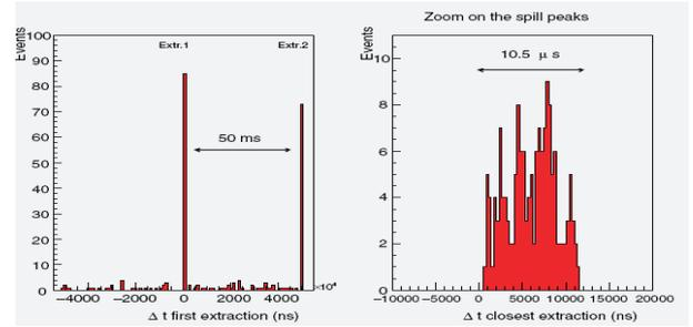
Figure 2: CNGS beam time structure seen in OPERA
