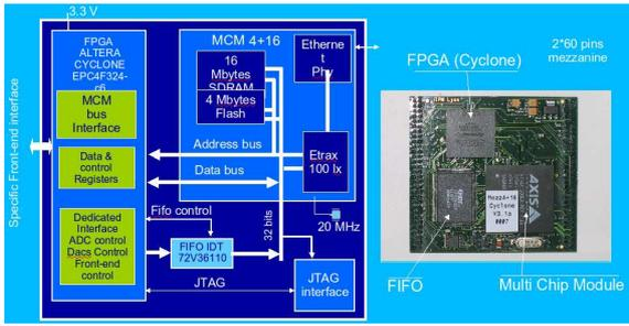
Figure 1: Ethernet Controller Module: schematics and physical view.
