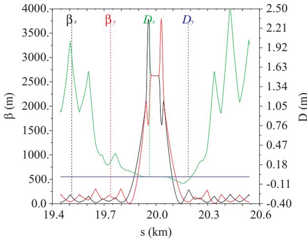
Figure 2: Beam 1 Optical functions for  $\beta^* = 2625$  m.
