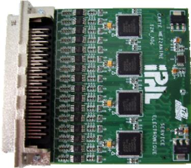
Fig. 4 Analog mezzanine board with 32 ADC channels
