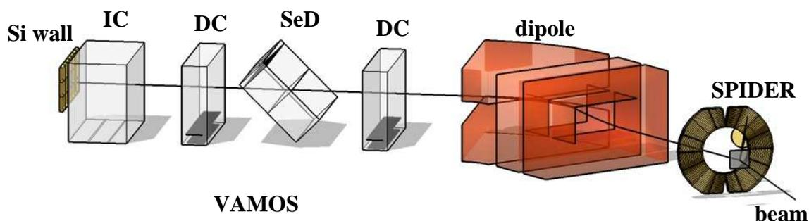
**FIGURE 1.** Experimental set-up. The VAMOS spectrometer and associated detectors are depicted in the figure. The dE-E telescope SPIDER is placed between the target (in grey) and the magnets of the spectrometer (in red)
