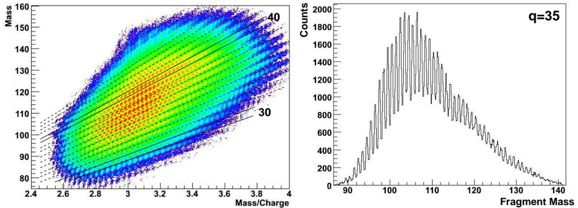
**FIGURE 4.** Fragment-A identification in VAMOS. Left panel:  $A$ - $A/q$  correlation. The dashed lines separate  $A$ - $A/q$  groups of fragments with the same charge state  $q$ . Right panel:  $A$  distribution of a single  $q$ . The distribution is obtained with  $A = q \times A/q$ . The shape of the distribution is due to the addition of different sets of data not yet normalized.
