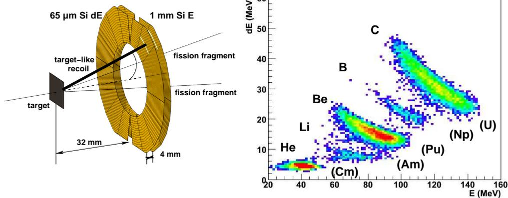
**FIGURE 2.** Left panel: Schematic drawing of the SPIDER-detector ensemble. Right Panel: Identification of target-like recoil in SPIDER. Correlation between dE-E shows the different recoil species produced in inelastic and transfer reactions. The corresponding fissioning elements are indicated in parenthesis.
