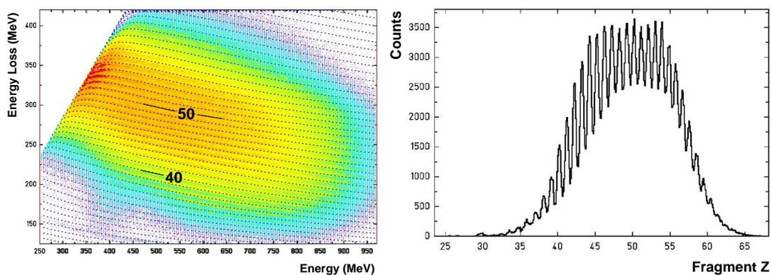
**FIGURE 3.** Fragment-Z identification in VAMOS. Left panel: dE-E correlation. The dashed lines correspond to the analytical description of dE-E correlation for each Z. Right panel: Z projection along the analytical lines. The shape of the distribution is due to the addition of different sets of data not yet normalized.
