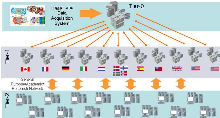
Figure 3: The LHC distributed computing model
