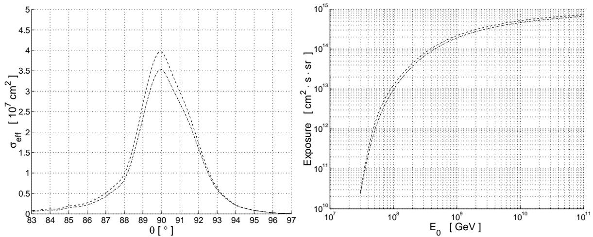
Figure 3: *Left*: effective surface at the trigger level as a function of the incoming  $\nu_\tau$  angle with the local vertical for  $10^{19}$  GeV  $\nu_\tau$ . *Right*: expected exposure in one year of data taking as function of the incident neutrino energy. The different curves correspond to triggers requiring 3 or 4 coincident antennas.
