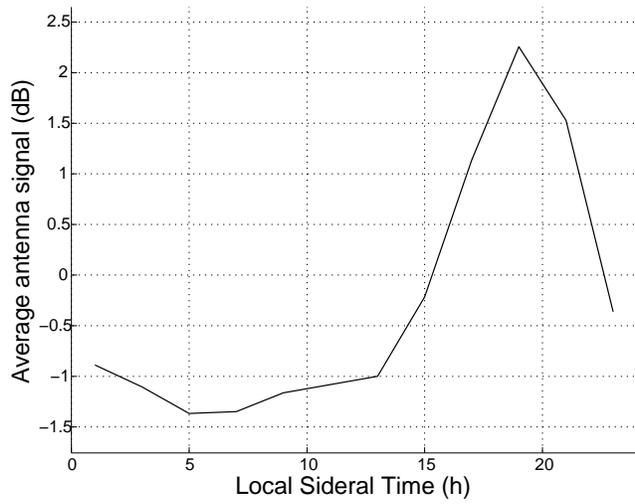
Figure 1: *Left*: average Fourier transform of the background noise for a 21CMA antenna. *Right*: antenna signal averaged over 15 hours of data taking as a function of the local sideral time, peaking to the galactic radio emission.
