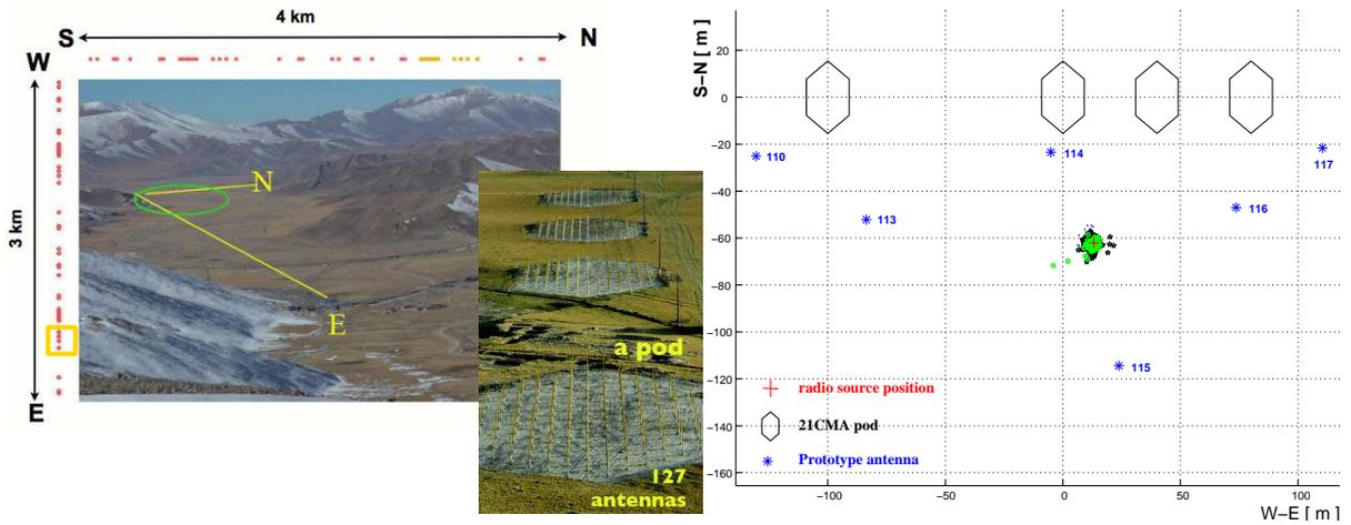
Figure 2: *Left*: the positions of the 81 pods in the two valley are shown (the red dots). The 6 pods housing our supplementary antennas are highlighted by the yellow rectangle. *Middle*: a close view of the pods. *Right*: the position of the six antennas (blue stars), the position of the car used as radio source (red cross) and the reconstructed origin of the signal (green and black points).
