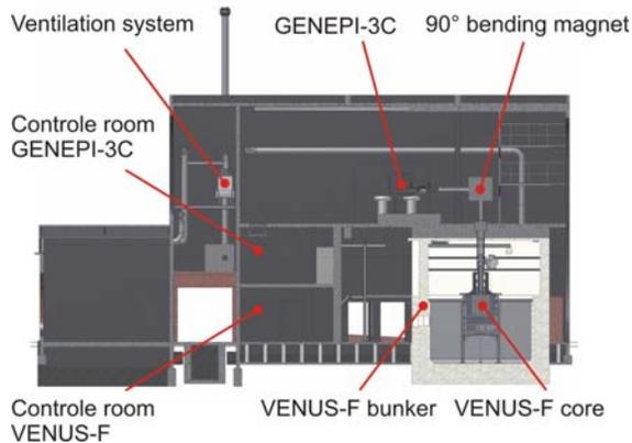
Fig. 3. Side view of the modified VENUS facility.
