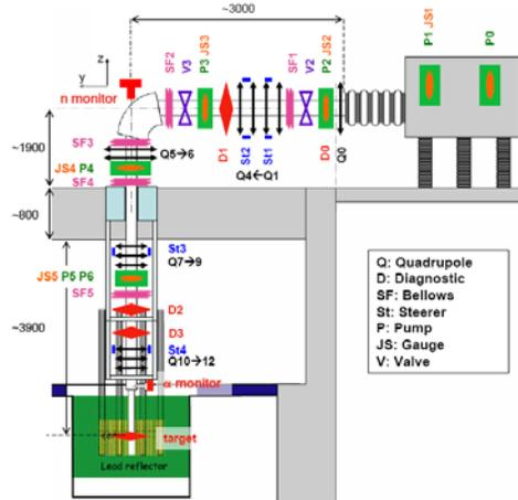
Fig. 5. Layout of the GENEPI-3C beam line components.
