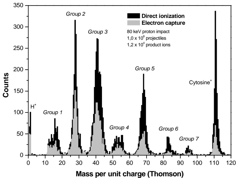
**Fig. 5:** Mass spectrum for proton impact ionization of thymine ( $C_5H_6N_2O_2$ , 126 amu) by electron capture and by direct ionization at 80 keV. The main ions expected to account for the peaks are listed in table 4.
