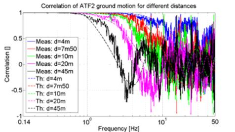
Figure 2: Measured correlation for several distances from the IP and theoretical one fitted on measurements.
