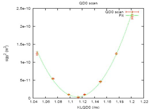
Figure 4: Vertical beam size as a function of KLQD0.
