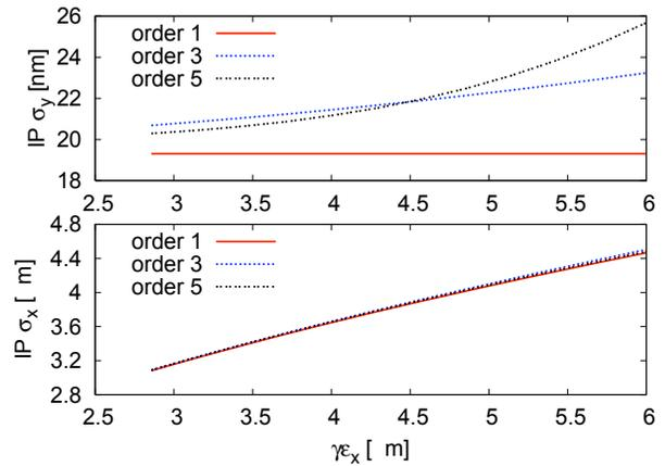
Figure 7: (top): Vertical beam size  $\sigma_y$  at the IP versus horizontal emittance for three different orders:quadrupolar, octupolar and dodecapolar. (bottom): Horizontal beam size  $\sigma_x$  at the IP versus horizontal emittance for the same orders.
