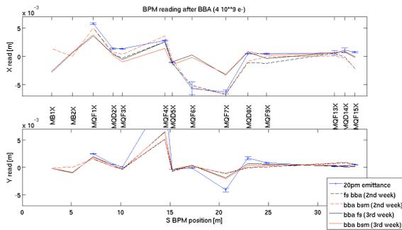
Figure 2: Monitoring beam position readings after BBA
