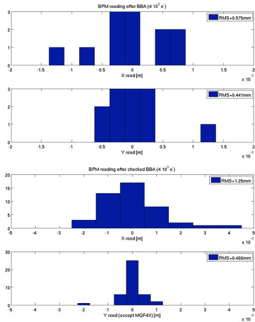
Figure 3: Spread of BPM readings after successive BBAs around mean values, for BPMs where careful BBA was done (upper two plots) and where it was only checked (lower two plots).
