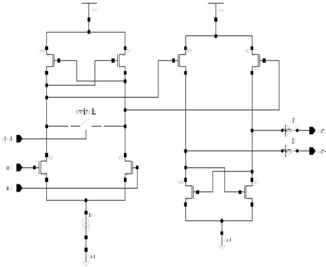
Figure 6: The diagram of the latched comparator
