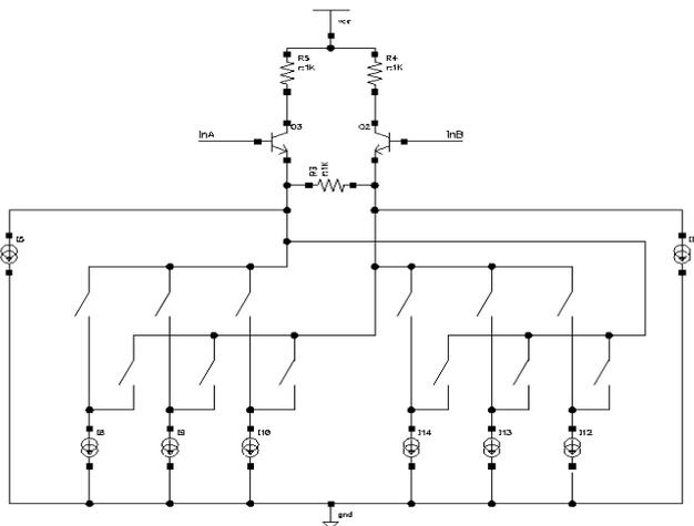
Figure 4: The subtractor structure, with the gain 2 differential amplifier and the current DAC structure. Depending on the results of the comparisons, the generators are distributed separately on one of the two branches.
