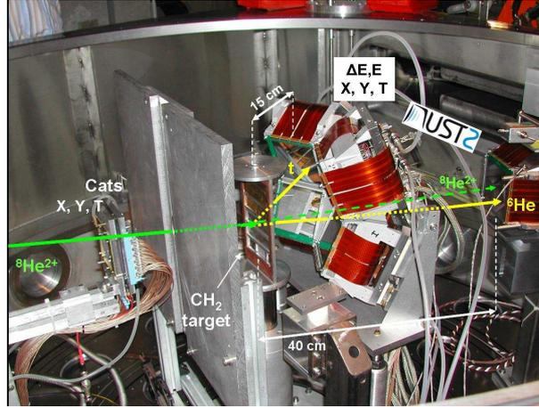
**Fig. 1:** Experimental set-up including one of the two beam detectors CATS, the array of 4 MUST2 telescope modules located at forward angles at 15 cm from the target, and the 5<sup>th</sup> telescope used at 0 degrees at 40 cm from the target (it appears rotated in this picture). An additional plastic scintillator (2 cm<sup>2</sup>) was located at 0 degrees in front of the 5<sup>th</sup> telescope.
