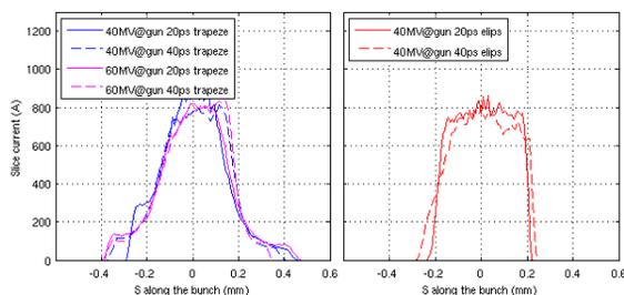
Figure 5: Current profile after compression to 800 A.
