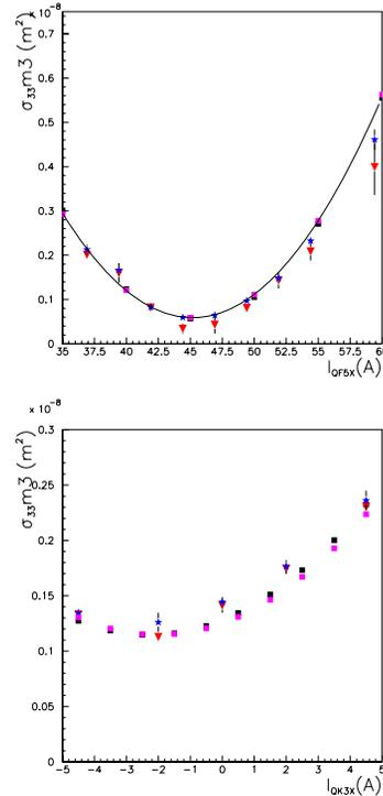
Figure 3:  $\sigma_{33}$  as function of QF5X (top) and QK3X (down) strength at MW3X. Blue stars correspond to the measured beam sizes, red triangles to the beam sizes corrected from the dispersion. The black and pink squares correspond to the simulated beam sizes using a coupling source, respectively at QM7 and both QM7 and BS1X.
