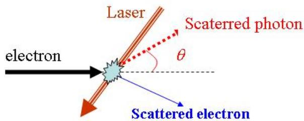
**Fig. 1.** Schematic view of the laser-electron Compton Scattering.
