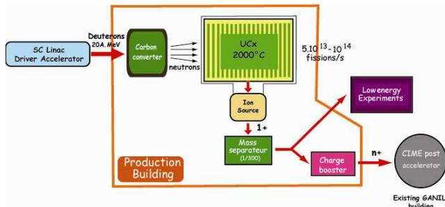
Figure 2 : RIB Production technique in Spiral 2
