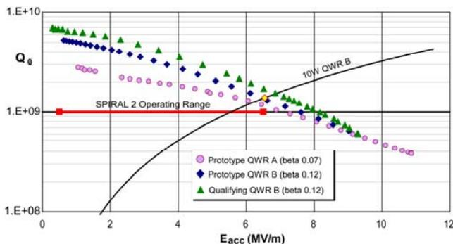
Figure 11: QWR performances of the Spiral 2 prototypes
