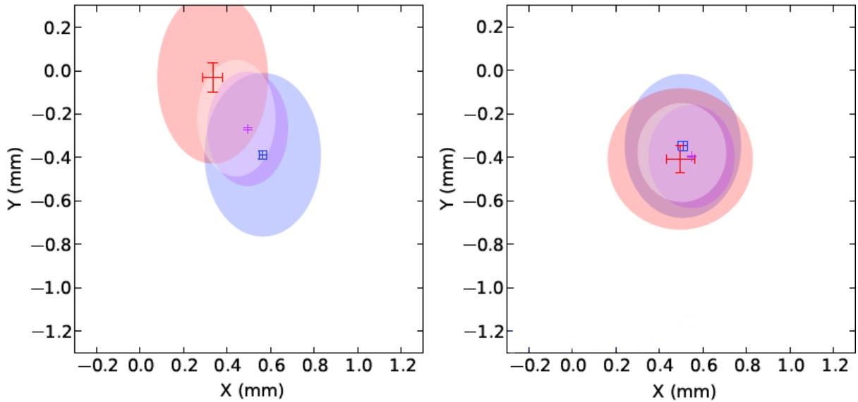
Figure 5: Observed beam positions and sizes at  $z = 0$  before and after beam adjustments (mini scan). The colors have the following meaning: blue - beam1, red - beam2, light grey - predicted luminous region, purple - measured luminous region.
