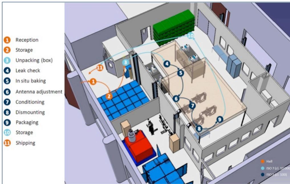
Figure 1: Complete process for RF conditioning of XFEL FPC at LAL.
