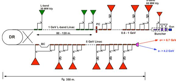
Figure 3: RF layout of the SuperB Injector.
