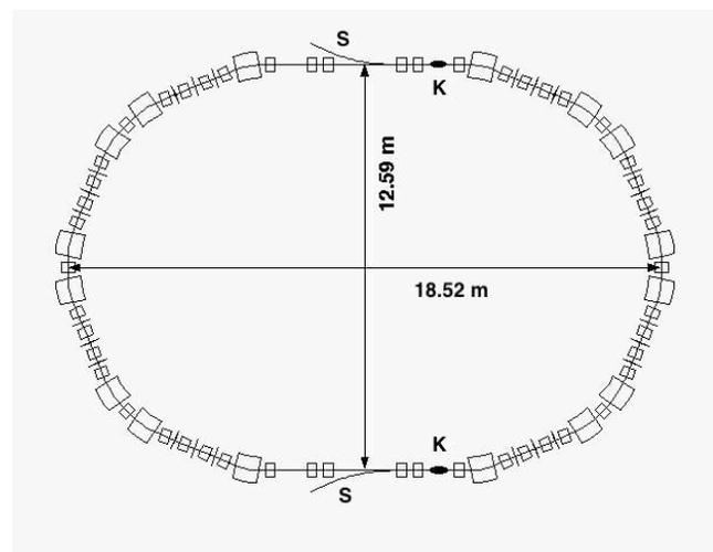
Figure 4: Damping ring layout.
