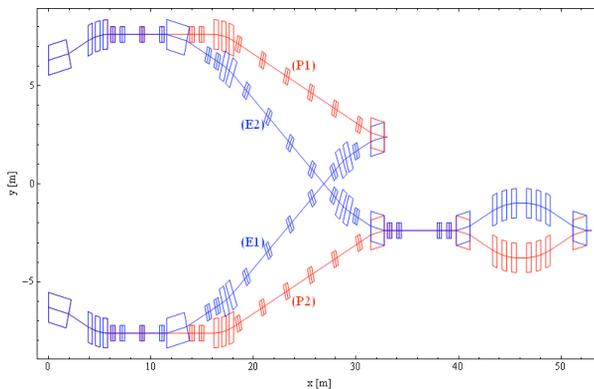
Figure 6: Layout of the transfer lines. Positron beams are red, electron beams blue.
