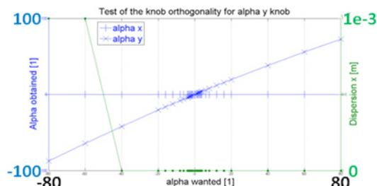
Figure 3: Linearity and orthogonality test (with MAD) of the  $\alpha_y$  multiknob based on QD0FF, QF1FF and QF9BFF
