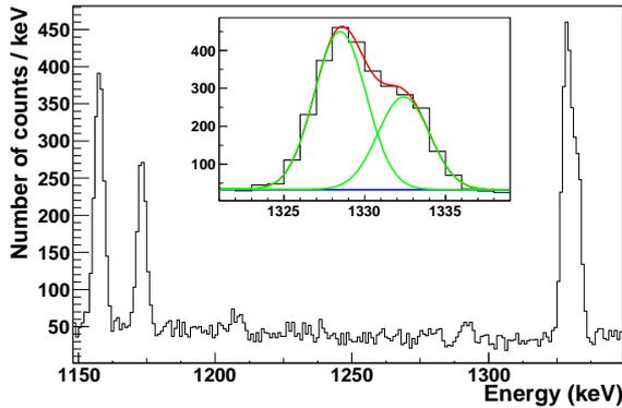
FIG. 2: Part of the delayed gamma energy spectrum following the implantation of  $^{44}\text{S}$  nuclei. Peaks from the  $\beta$  decay of  $^{44}\text{K}$  (1158 keV) and  $^{60}\text{Co}$  (1173 and 1332.5 keV) are identified, the latter overlapping with the 1329 keV  $2_1^+ \rightarrow 0_1^+$  transition of  $^{44}\text{S}$ . The deconvolution of this doublet is shown in the insert.
